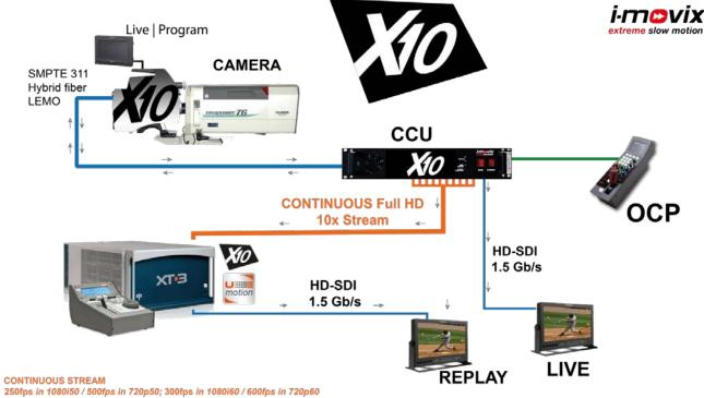
The X10 camera is linked to the XT3 production server via the I-MOVIX® CCU, which handles communication between the camera and the server (through RS-422 link) and between the camera and its OCP (for camera setup). Ultra Motion footage coming from X10 is recorded on the XT3 server and can be accessed, replayed (at variable speeds) or processed as usual with the EVS remoteLSM
